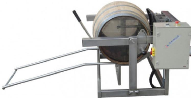
In this model, a counterweight system facilitates the lifting of the barrel to place it in the washing position, and returns it to its loading and unloading position.
